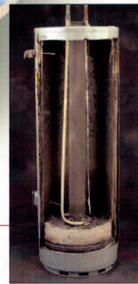
Example of mineral buildup in an unprotected water heater.
